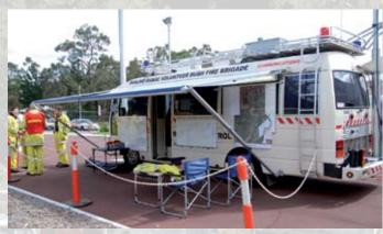
Communications is provided through two-way radios, fax, mobile and satellite phones. All radio traffic is recorded on a 4 channel tape recorder. Additional equipment carried includes a Mobile Duplex Repeater.
